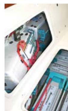
Six converters – one each for the six propulsion batteries in series
