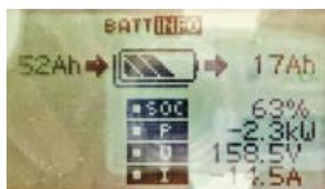
Using a little current to make the props turn faster while generating, in this case 17Ah, the power generated is increased significantly, 52Ah here. Software is being developed to optimise the balance automatically
