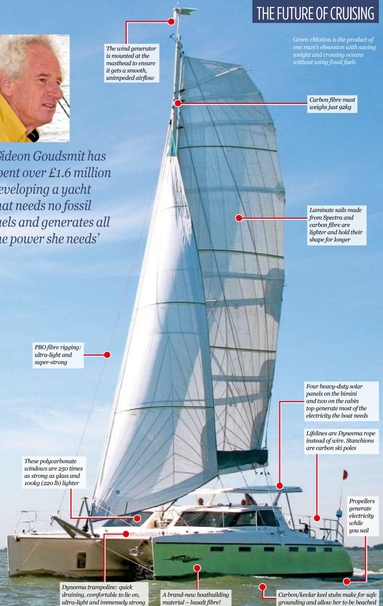
The wind generator is mounted at the masthead to ensure it gets a smooth, unimpeded airflow
