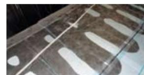
*Using vacuum infusion more than halves the amount of resin required, saving almost one tonne on a 45ft catamaran*
