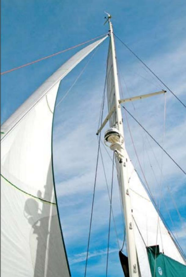
**Sails** The sails are Spectra and carbon fibre cruising laminates, made by North. Gideon says these offered the best combination of light weight, longevity and shape retention, which is essential for efficient sailing.
