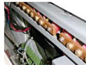
The bus bars will be downsized. The green dump resistors dissipate excess power
